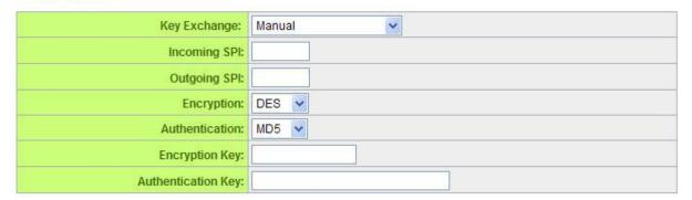
If the Manual mode is selected, users need to set encryption key manually without negotiation.
