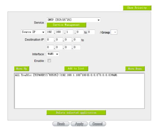
Example 2: How do I set up Auto Load Balance Mode to keep Intranet IP 192.168.1.150 ~ 200 from going through WAN2 when the destination port is Port 80?
