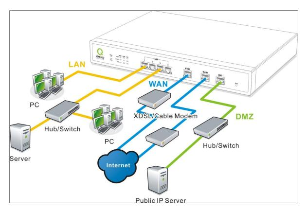
**WAN connection**: A WAN port can be connected with xDSL Modem, Fiber Modem, Switching Hub, or through an external router to connect to the Internet.
