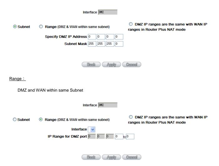
**IP Range:** Input the IP range located at the DMZ port.
