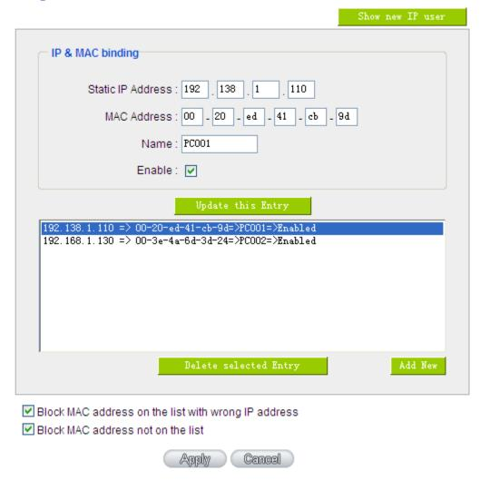
Though these basic operations can help solve the problem but Qno's technical engineers suggest that further measures should be taken to prevent the ARP attack.
