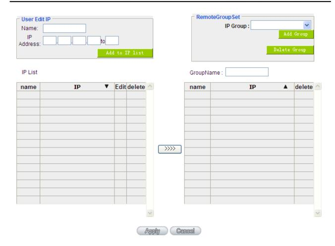
It is the same setting methods. You should set the IP address or the range of remote IP from the left side first, and choose to add IP address information from the left side into the remote group.
