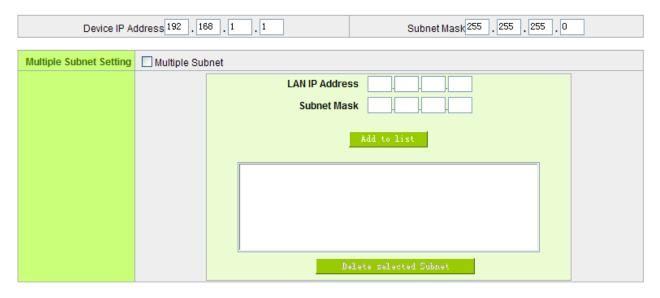
This function enables users to input IP segments that differ from the router network segment to the multi-net segment configuration; the Internet will then be directly accessible. In other words, if there are already different IP segment groups in the Intranet, the Internet is still accessible without making any
