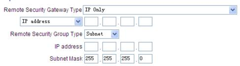
This remote gateway authentication type (Remote Security Gateway Type) must be identical to the remotely-connected local security gateway authentication type (Local Security Gateway Type).
