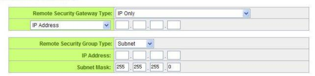
This remote gateway authentication type (Remote Security Gateway Type) must be identical to the remotely-connected local security gateway authentication type (Local Security Gateway Type).
