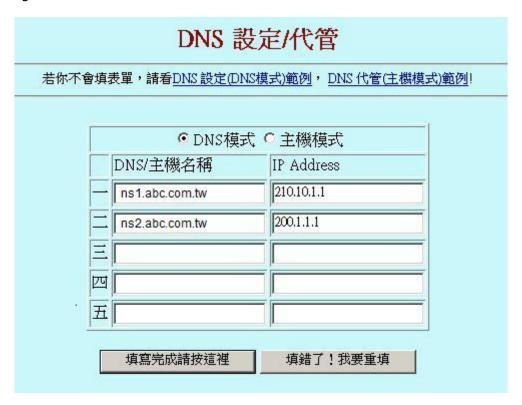
Choose DNS mode, and then fill in the Host name and corresponding IP address of WAN1 and WAN2. Press "Finish" button, the setting will be effective in 24 hours.
