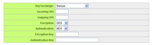
If there is any encryption mechanism, the encryption mechanism of these two VPN tunnels must be identical in order to create connection. And the transmission data must be encrypted with IPSec key, which is known as the encryption "key". The device provides the following two encrypted Key Managements. They are Manual and IKE automatic encryption mode- IKE with Preshared Key (automatic). By using the drop down menu, select the desired encryption mode as illustrated below.
