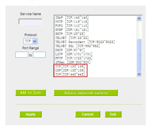
b. Use the "Access Rule" in the firewall and set to block these three ports.
